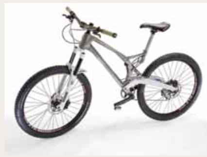
Renishaw, is UK's only manufacturer of a metal-based additive manufacturing machine that prints parts. It collaborated with a leading British bicycle design and manufacturing company to create the world's first 3D printed metal bike frame. Empire Cycles designed the mountain bike to take advantage of Renishaw's additive manufacturing technology, allowing them to create a titanium frame that would be both strong and light using topological optimisa-
